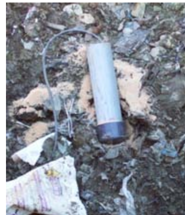
Figure 2-8 Installation of Thermocouples in Cell 6
