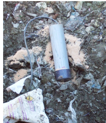
Figure 2-9 Installation of Thermocouples in Cell 6
