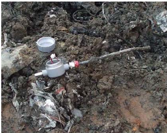
Figure 2-9 Installation of Thermocouples in Cell 6
