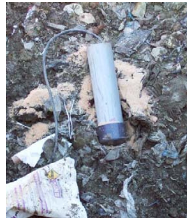
Figure 2-9 Installation of Thermocouples in Cell 6
